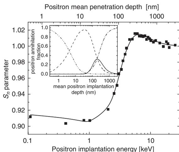
Fig. 1.  $S_n$  versus positron implantation energy and positron mean implantation depth (upper axis). The continuous line is the best fit with the diffusion model (Brusa et al., 2000). In the inset the positron annihilation probability:  $f_s$  at the surface (dash-dot-dot);  $f_d$  in the surface defects (dash);  $f_c$  in the cavities (continuous line);  $f_b$  in the bulk (dash-dot).
