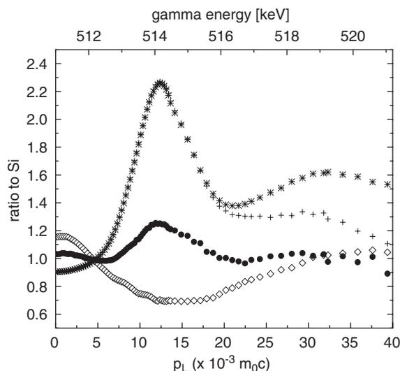
Fig. 2. Ratio curves to bulk Si. Full dots, ratio of the annihilation peak as measured at 6 keV. Extracted characteristic ratio curve for surface defects (crosses), silicon dioxide at the surface (stars), cavities (open diamond).  $p_L$  is the longitudinal momentum of the positron–electron pair.
