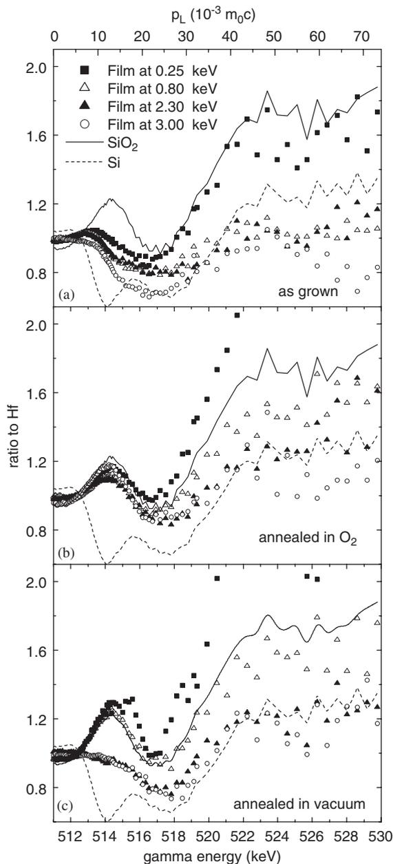
Fig. 4. Ratio curves to bulk Hf. Ratio of the annihilation peak as measured at 0.25, 0.8, 2.3 and 3.0 keV positron implantation energies. The ratio curves for  $\text{SiO}_2$  and Si are also presented. (a) As grown film; (b) film annealed in  $\text{O}_2$ ; (c) film annealed in vacuum.
