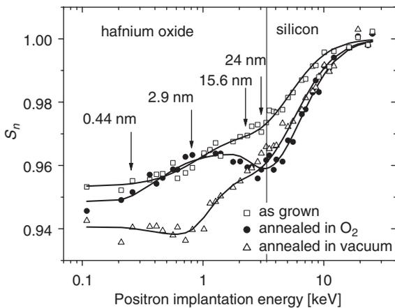
Fig. 3.  $S_n$  versus positron implantation energy for hafnium oxide films: as-grown, annealed in vacuum and annealed in O<sub>2</sub>. The continuous lines are best fit with VEPFIT (van Veen et al., 1990).
