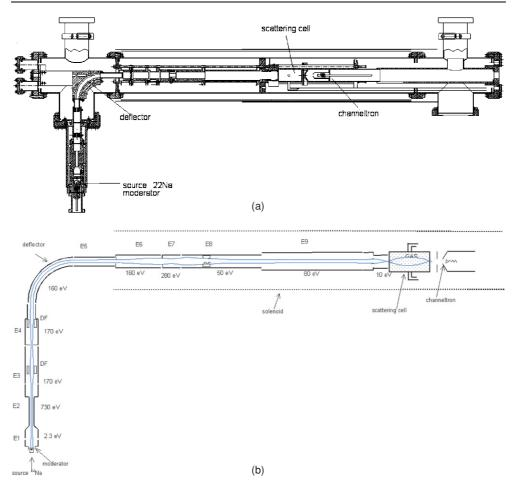
**Figure 1.** Schematic drawings of the apparatus. (a) Vacuum chambers, connections to pumps and technical drawings of the optics. (b) Scheme of the electron optics:  $E_i$  stand for electrodes, DF are deflection plates. Numbers (in eV) indicate kinetic energies of positrons at given points.
