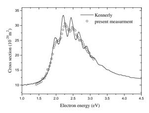
Fig. 4. Total cross section for electron scattering on N<sub>2</sub>: the present measurements are compared with the data of Kennerly (1980). This measurement allows to determine the apparatus energy resolution as  $(\Delta E/E \sim 130/2 \text{ meV/eV})$ .
