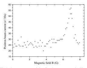
Fig. 3. Apparatus transmission function as measured with a positron beam: note the scale change. The position of the peak is different from the position in Fig. 2 due to the different emission energies.
