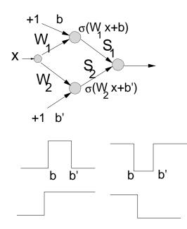
Fig. 1. Construction of a linguistic unit converting continuous inputs to linguistic variables.
