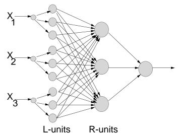
Fig. 2. Structure of the network for rule extraction and feature selection. *L*-units convert continuous inputs into linguistic variables, *R*-units form the rules.
