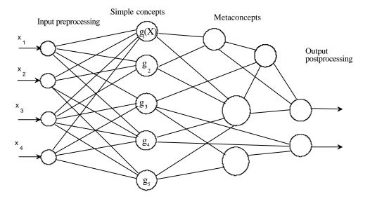
Example of the network realizing Floating Gaussian Mapping
