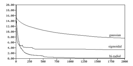
Figure 5: Comparison of the summed squared errors for different transfer functions: gaussian (Eq. 10), sigmoidal (Eq. 15) and bi-radial function (Eq. 18) used in the same RBF net during 2000 epochs.
