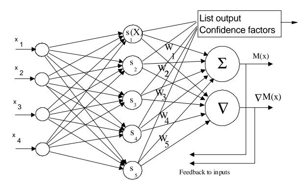
Fig. 2 Example of a network realizing the Feature Space Mapping (FSM) model.
