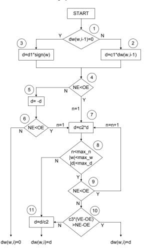
Fig. 4. Sketch of the Variable Step Search algorithm determining a single weight value in one training cycle.
