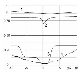
Fig. 2. Typical error surface crossections in the direction of: (1) hidden weight at the beginning of the training; (2) output weight at the beginning of the training, (3) output weight at the end of the training, (4) hidden weight at the end of the training.
