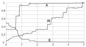
Fig. 7. MSE error (E), classification accuracy on the training set (A) and normalized weight ||W(i)||/||W(5)|| vector length (W) during the first 5 training cycles for the Iris (4-4-3) network
