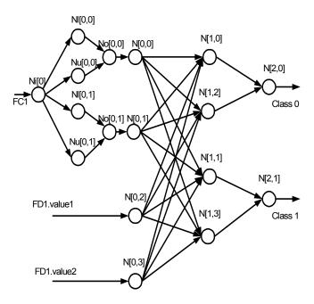
Fig. 1. SMLP Network Diagram, with some pre-processing L-units shown for FC1 feature
