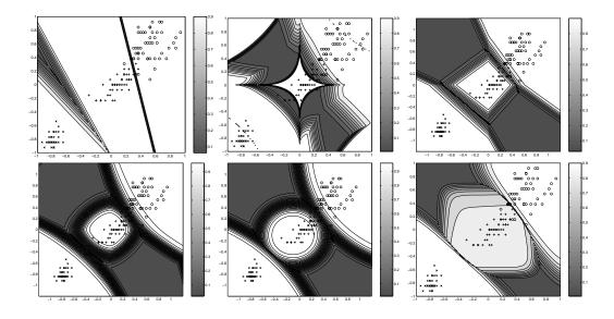
Figure 6: Shapes of decision borders in the Iris case for standard MLP (3 neurons) and an MLP network in the extended space with vectors renormalized using Minkovsky metric,  $\alpha = 0.5, 1.0, 1.5, 2.0$  and 7.0.
