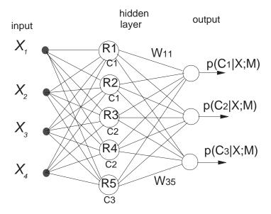
Figure 2: Network generalization of the k-NN method. The hidden nodes compute distances to reference vectors and return k values of class labels associated with the nodes, while the output nodes compute probabilities.
