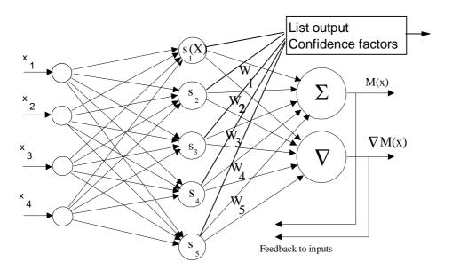
Fig. 2. Feature Space Mapping network module. The whole system is composed from several such modules specializing in classification of different type of data and contributing to the final system identification performed by the reasoning module.
